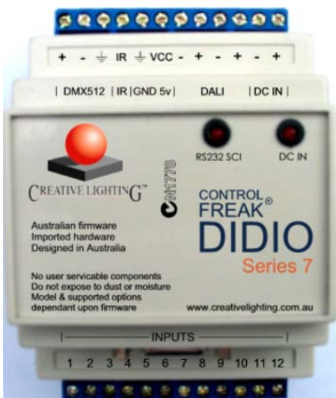
DIDIO – a convenient din mount combination of integral modules of DALI power supply 21vdc 245mA, SCI Serial Communications Interface, and DALI Scene Controller with up to 12 i/o lines
